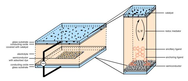
**Figure 1:** Structure of a dye-sensitized solar cell with zoom-in example for investigated copper(I) dye-sensitized solar cells.
